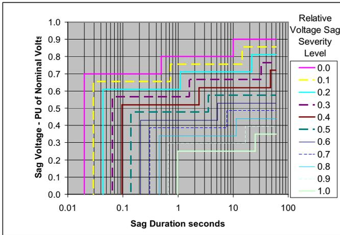
Fig. 9. Sag SAIFI Model – Voltage Sag Severity Levels
