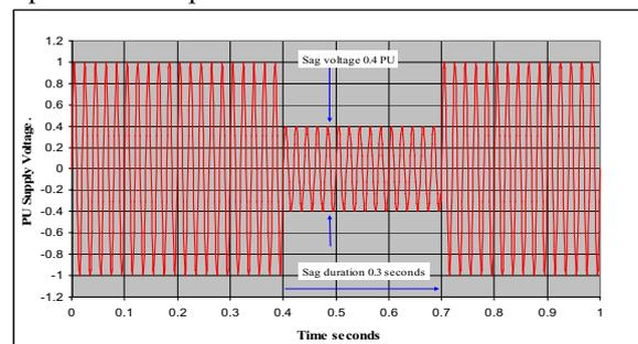
Fig. 1. Typical voltage sag waveform
