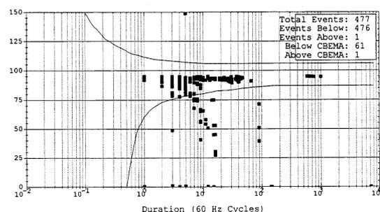
Fig. 2. Comparison of voltage sags with the CBEMA curve
