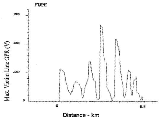
Figure 5: Coating Stress Voltage with insulating joints
