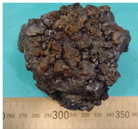
Figure 5: A piece of cold sinter prepared from fine manganese ore and manganese furnace dust
