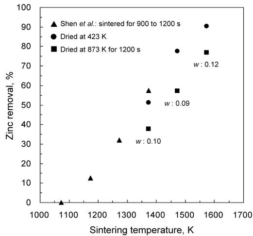
**Fig. 4.** Effect of the sintering temperature on zinc removal. Samples with initial thickness of 20 mm were sintered for 1 200 s.
