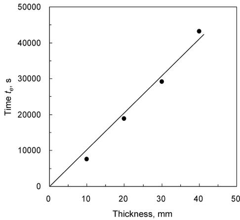
Fig. 9. Time needed to fully dry dust samples of different thickness at 423 K.
