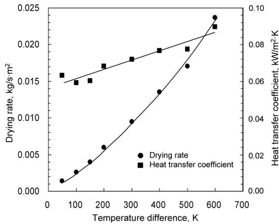
Fig. 12. Rate constant and heat transfer coefficient in the process of dust drying at different temperatures. Difference between the furnace and sample temperatures is taken at drying stage with constant rate.
