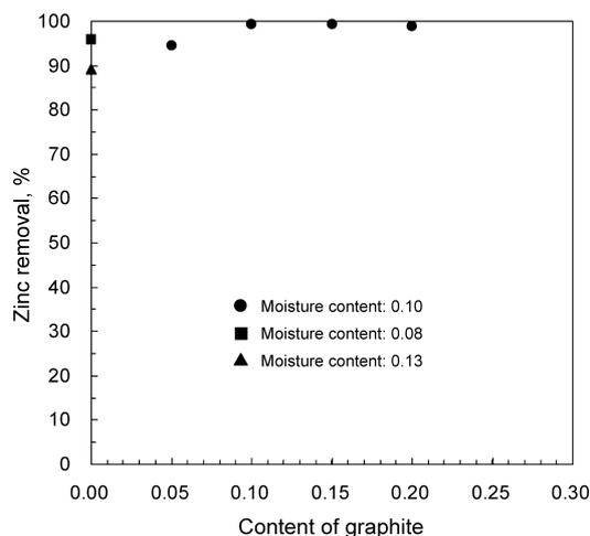
**Fig. 7.** Effect of addition of graphite on zinc removal. Sample thickness was 20 mm. Sintering was carried out at 1573 K for 1200 s.
