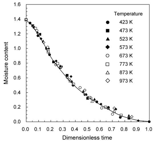
Fig. 11. Relationship between the moisture content in the manganese dust and dimensionless time.
