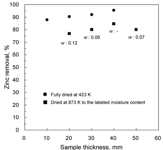
**Fig. 6.** Relationship between zinc removal and the initial thickness of samples. The samples were sintered at 1 573 K for 1 200 s.
