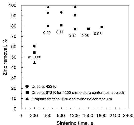
**Fig. 3.** Zinc removal in process of sintering of manganese dust at 1 573 K. The initial thickness of samples was 20 mm.
