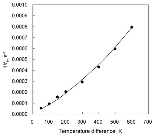
Fig. 10. Time needed to fully dry a 20 mm thick sample at different temperatures. Difference between the furnace and sample temperatures is taken at drying stage with constant rate.
