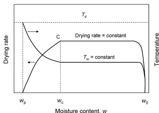
**Fig. 8.** Change of drying rate and material temperature with moisture content.
