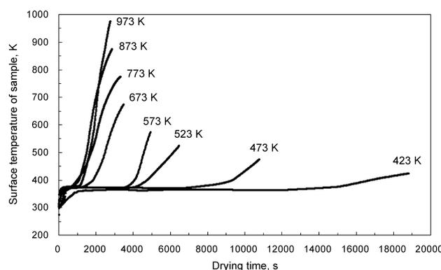
**Fig. 2.** Surface temperature of samples of manganese furnace dust in process of drying at different temperatures.
