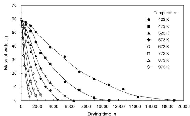
**Fig. 1.** Drying of manganese dust at different temperatures. Sample thickness was 20 mm, surface area  $3.6 \times 10^{-3} \text{ m}^2$ .
