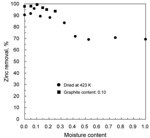
**Fig. 5.** Effect of the initial moisture content on zinc removal. Samples with initial thickness of 20 mm were sintered at 1 573 K for 1 200 s.
