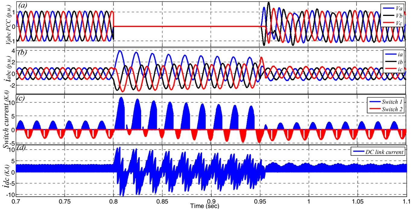
Fig. 3. Simulation results for the LLLG fault at point F without the proposed DLFC. (a) three-phase voltages at point F ( $V_a$ ,  $V_b$  and  $V_c$ ), (b) three-phase output current of the VSI ( $i_a$ ,  $i_b$  and  $i_c$ ), (c)  $A$ -phase switch current of the inverter (switch 1 and switch 2), (d) the DC link current ( $i_{dc}$ ).
