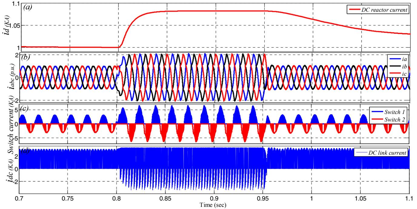
Figure 4. Simulation results for the LLLG fault at point F when the proposed DLFC is employed: (a) the DC reactor current ( $i_d$ ), (b) three-phase output current of the VSI ( $i_a$ ,  $i_b$  and  $i_c$ ), (c)  $A$ -phase switch current of the inverter (Switch 1 and switch 2), (d) DC link current ( $i_{dc}$ ).
