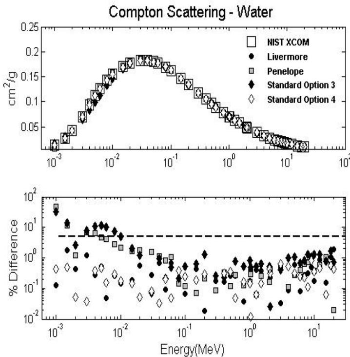
**Figure 2.** Energy dependence of the Compton scattering attenuation coefficient in water for different Geant4 10.1 models and NIST XCOM data [12] (top); difference between Geant4 and NIST XCOM (bottom). The dashed line is the maximum uncertainty of NIST XCOM.
