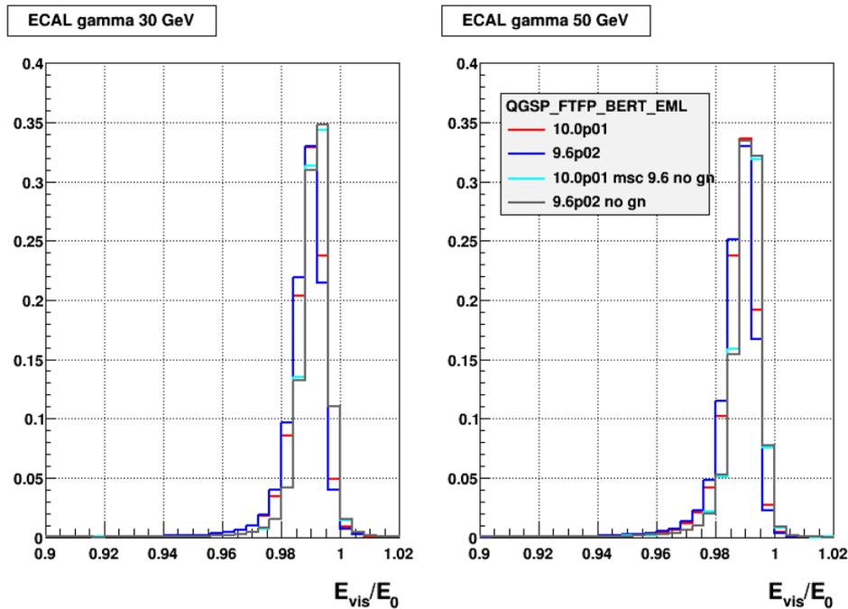
**Figure 4.** Response of CMS type simplified combined calorimeter (ECAL + HCAL) for 30 GeV and 50 GeV electron beams for different variants of EM physics configuration.
