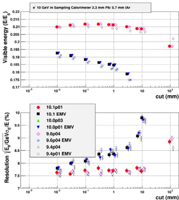
**Figure 3.** Response and resolution of ATLAS-barrel type simplified sampling calorimeter as a function of Geant4 cut in range. Different markers correspond to different Geant4 versions and EM physics options.
