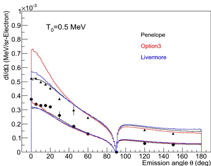
**Figure 7.** Angular distribution of the bremsstrahlung yield of 0.5-MeV electrons impinging on thick targets of Al (0.548 g/cm<sup>2</sup>) and Fe (0.257 g/cm<sup>2</sup>). Points are experimental data from Ref. [15] (circles - Al target, triangles - Fe target). Histograms are the predictions from the Geant4 simulation.
