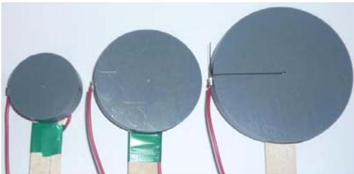
Fig. 7. Circular contact surfaces used (20mm, 30 mm, and 40 mm in radius).
