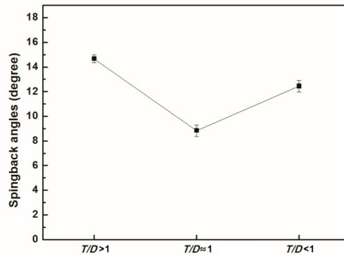
**Fig. 5.** Springback angles for each  $T/D$  ratio
