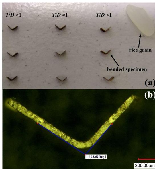
**Fig. 4.** Photo of (a) bended specimens and (b) a measured specimen under VHX-1000 KEYENCE.
