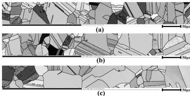
**Fig. 1.** Microstructures of annealed phosphor bronze foils: (a)  $T/D > 1$ , (b)  $T/D \approx 1$  and (c)  $T/D < 1$ .
