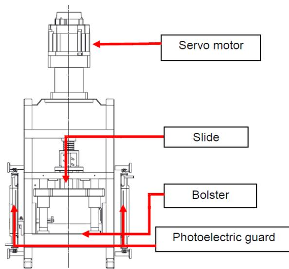
**Fig. 2.** Schematic of desk-top servo press machine DT-3AW.
