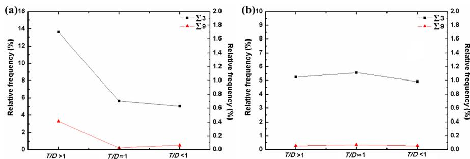
**Fig. 7.** (a) The frequencies of  $\Sigma 3$  and  $\Sigma 9$  twinning boundaries before bending, and (b) the frequencies of  $\Sigma 3$  and  $\Sigma 9$  twinning boundaries after bending.
