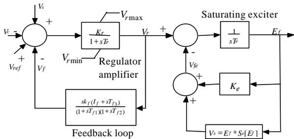
Fig.3: IEEE type AC5A Exciter system [9]
