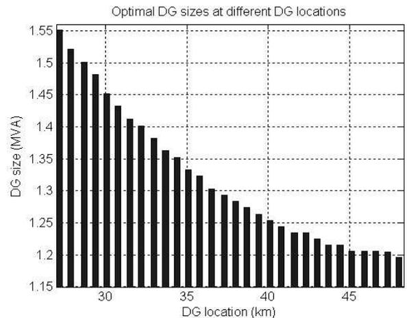
Figure 7: Optimal DG sizes for different DG locations
