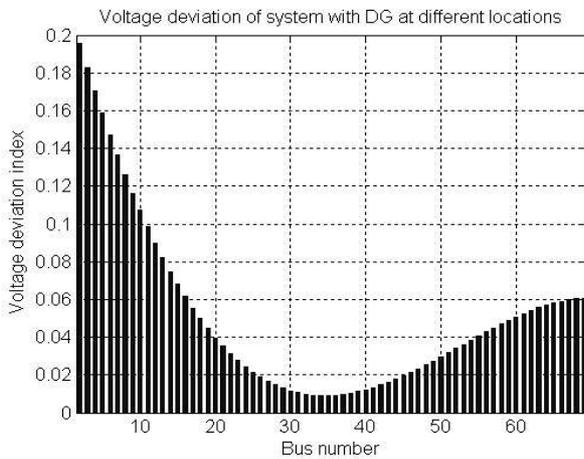
Figure 3: Voltage deviation with the 100% DG penetration
