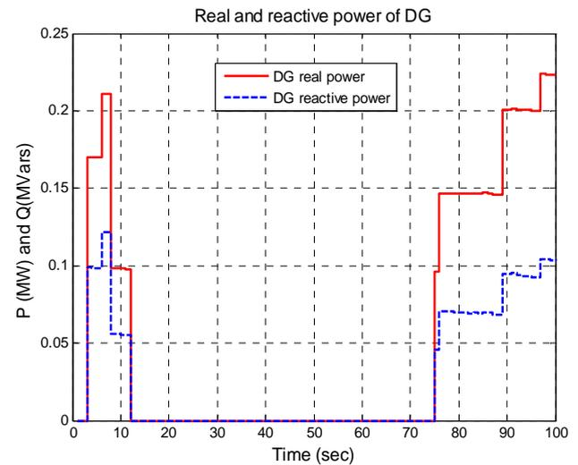
Figure 6: DG injection power with non-delayed DG
