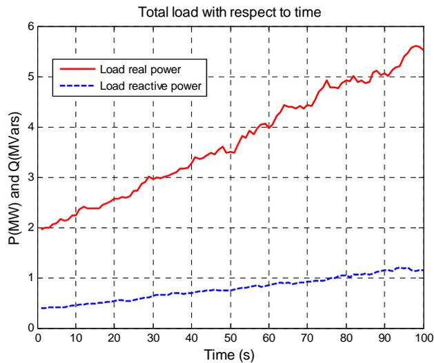
Figure 4: Total feeder active and reactive load profiles
