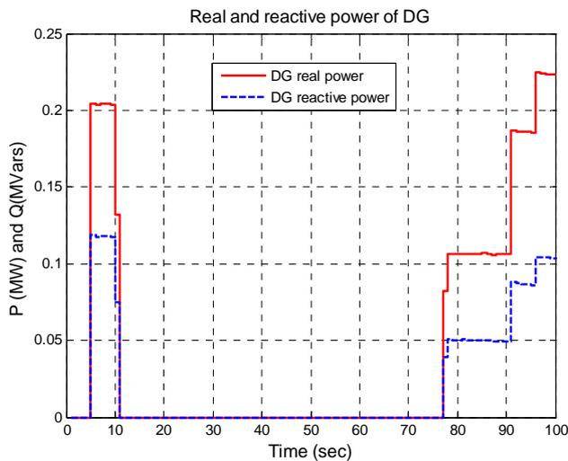
Figure 7: DG injection power with delayed DG
