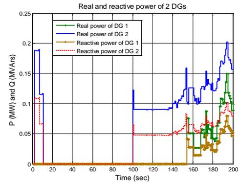
Figure 15: The DG response for non-communication voltage control
