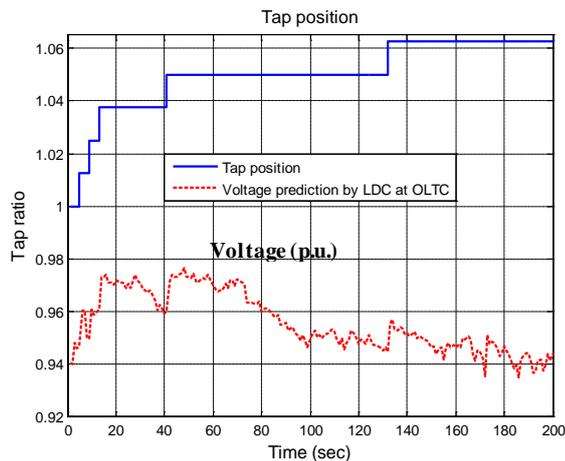
Figure 10: Tap position in case of delayed and non-delayed DG to support feeder load and voltage prediction at OLTC by the proposed tuning approach
