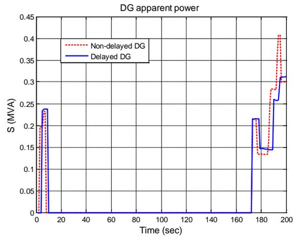
Figure 11: DG power injection with delayed and non-delayed DG
