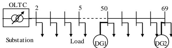
Figure 5: Diagram of a simplified test feeder
