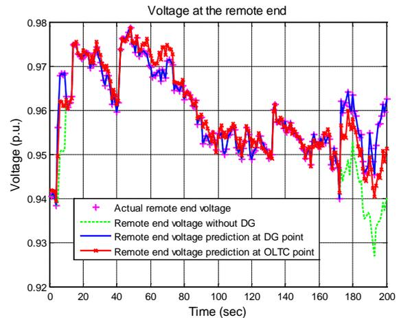
Figure 12: Remote end voltage with respect to time for the case of delayed DG
