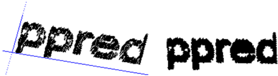
(a) Pixels determined to belong to the characters. (b) Final post-processed image.
