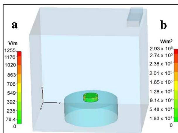
**Fig. 2 Modelling of (a) electric field (V/m) and (b) absorbed power ( $W/m^3$ ) is shown using CST Microwave Studio 3D Electromagnetic Simulation Software.**
