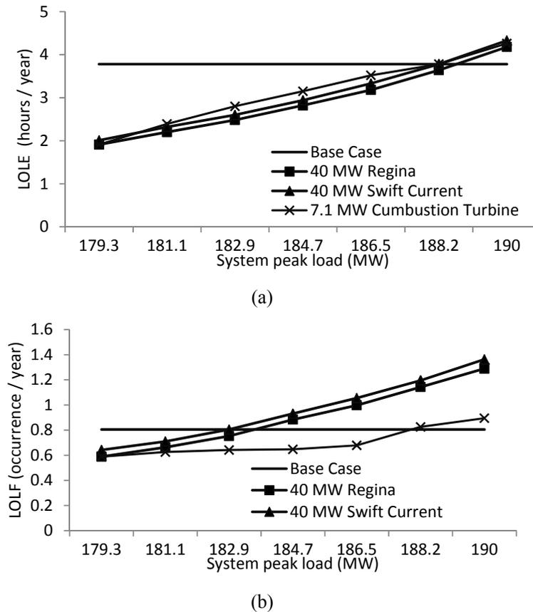
Fig. 4. ELCC obtained using LOLE and LOLF: (a) LOLE index; (b) LOLF index.
