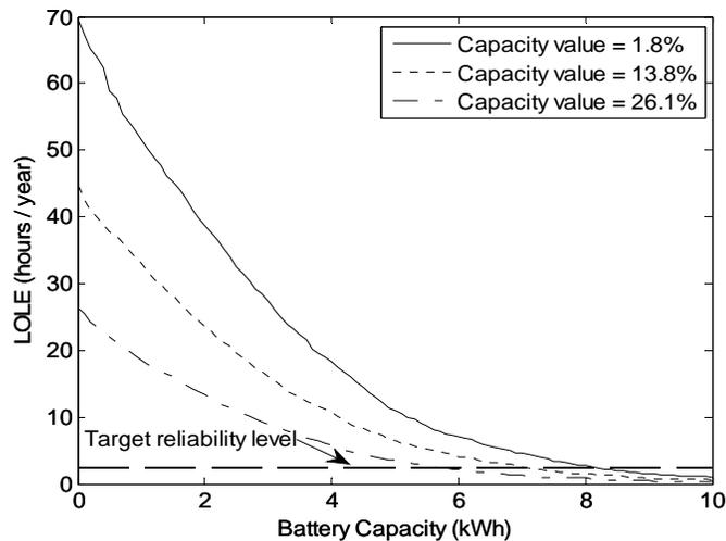
Fig. 3. Impact of storage on RAPS system reliability
