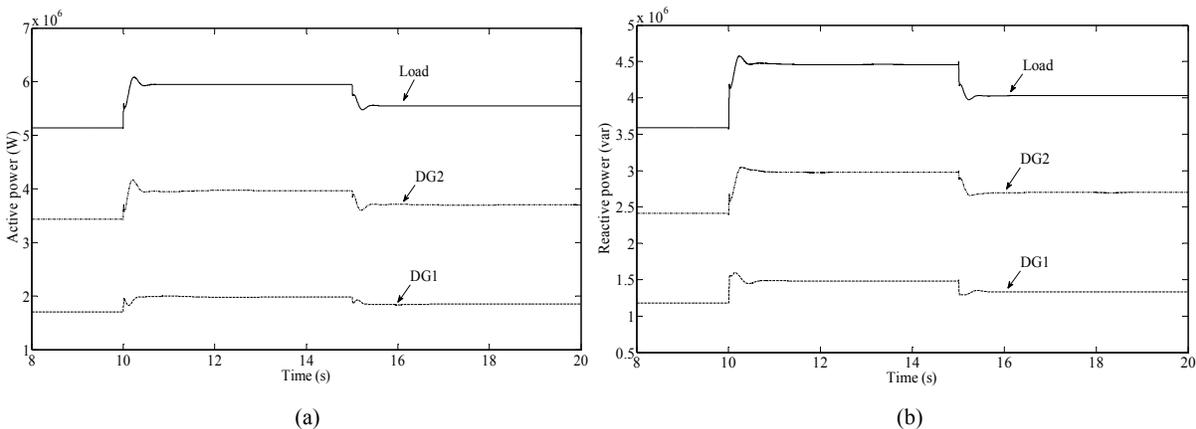
Fig.5. RAPS system with two conventional generators: a. Active power sharing. b. Reactive power sharing
