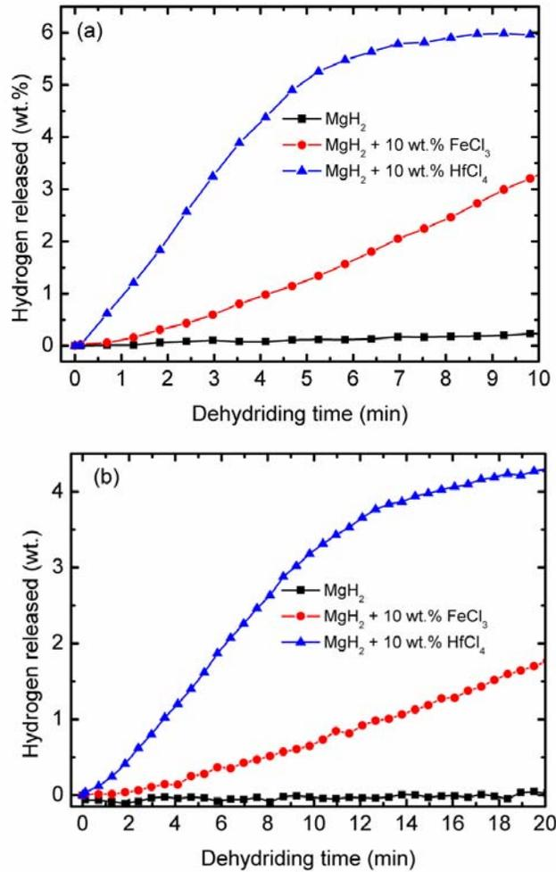
Fig. 3. Desorption kinetics measurements of MgH<sub>2</sub>, MgH<sub>2</sub> + 10 wt.% FeCl<sub>3</sub>, and MgH<sub>2</sub> + 10 wt.% HfCl<sub>4</sub> at (a) 300 °C and (b) 280 °C under vacuum.
