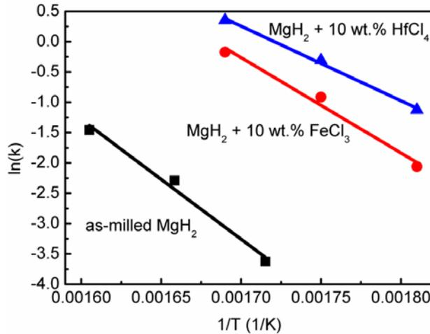
Fig. 4. Arrhenius plots of  $\ln(k)$  vs.  $1/T$  for as-milled  $MgH_2$ ,  $MgH_2 + 10$  wt.%  $FeCl_3$ , and  $MgH_2 + 10$  wt.%  $HfCl_4$ .
