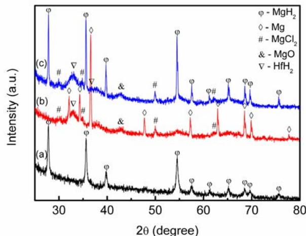
Fig. 11. X-ray diffraction patterns of the 50 wt.% HfCl<sub>4</sub>-doped MgH<sub>2</sub> (a) after milling, (b) after dehydrogenation and (c) after rehydrogenation.
