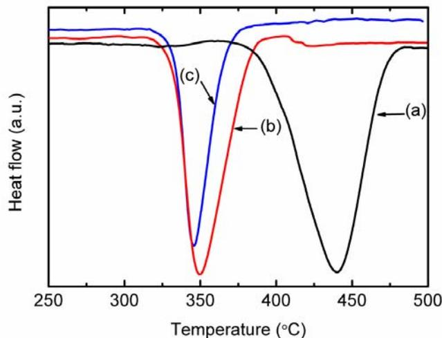
Fig. 2. DSC traces of (a) as-milled  $\text{MgH}_2$ , (b)  $\text{MgH}_2 + 10 \text{ wt.}\% \text{FeCl}_3$ , and (c)  $\text{MgH}_2 + 10 \text{ wt.}\% \text{HfCl}_4$ . Heating rate:  $15 \text{ }^\circ\text{C min}^{-1}$ , argon flow:  $30 \text{ ml/min}$ .
