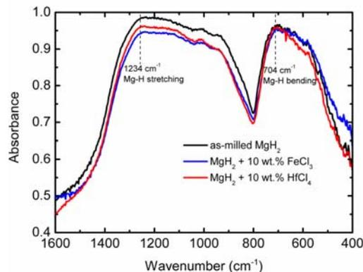
Fig. 9. FTIR spectra of as-milled  $\text{MgH}_2$ ,  $\text{MgH}_2 + 10 \text{ wt.}\% \text{ FeCl}_3$ , and  $\text{MgH}_2 + 10 \text{ wt.}\% \text{ HfCl}_4$ .
