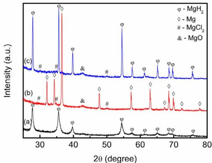
Fig. 8. X-ray diffraction patterns of the HfCl<sub>4</sub>-doped MgH<sub>2</sub> (a) after milling, (b) after dehydrogenation, and (c) after rehydrogenation.
