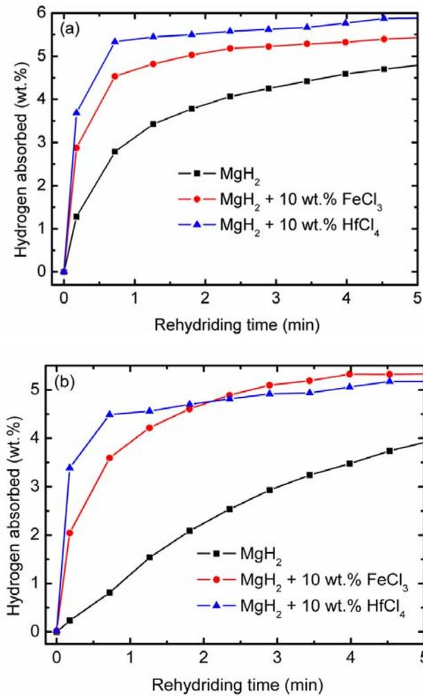
Fig. 5. Absorption kinetics measurement of MgH<sub>2</sub>, MgH<sub>2</sub> + 10 wt.% FeCl<sub>3</sub>, and MgH<sub>2</sub> + 10 wt.% HfCl<sub>4</sub> at (a) 300 °C and (b) 280 °C under 3 MPa hydrogen pressure.
