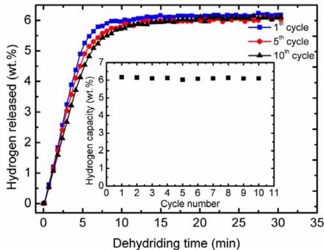
Fig. 6. The cycling performance of  $\text{MgH}_2 + 10 \text{ wt.}\% \text{ HfCl}_4$  at  $300 \text{ }^\circ\text{C}$  under vacuum after rehydrogenation at  $300 \text{ }^\circ\text{C}$  under 3 MPa hydrogen pressure. The main figure shows the hydrogen released in the 1<sup>st</sup>, 5<sup>th</sup>, and 10<sup>th</sup> cycles, while the inset shows the hydrogen capacity vs. cycle number.
