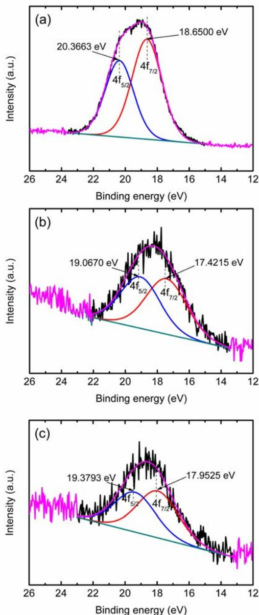
Fig. 10. XPS Hf 4f spectra with fitting results for pure HfCl<sub>4</sub> (a) and for MgH<sub>2</sub> + 10 wt.% HfCl<sub>4</sub> after (b) dehydrogenation and (c) rehydrogenation.
