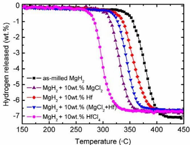
Fig. 12. Temperature-programmed desorption (TPD) patterns for the dehydrogenation of as-milled MgH<sub>2</sub>, and MgH<sub>2</sub> doped with 10 wt.% MgCl<sub>2</sub>, Hf, (MgCl<sub>2</sub>+Hf), and HfCl<sub>4</sub>.
