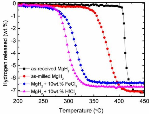
Fig. 1. Temperature-programmed desorption (TPD) patterns for the dehydrogenation of as-received  $\text{MgH}_2$ , as-milled  $\text{MgH}_2$ ,  $\text{MgH}_2 + 10 \text{ wt.}\% \text{FeCl}_3$ , and  $\text{MgH}_2 + 10 \text{ wt.}\% \text{HfCl}_4$ .
