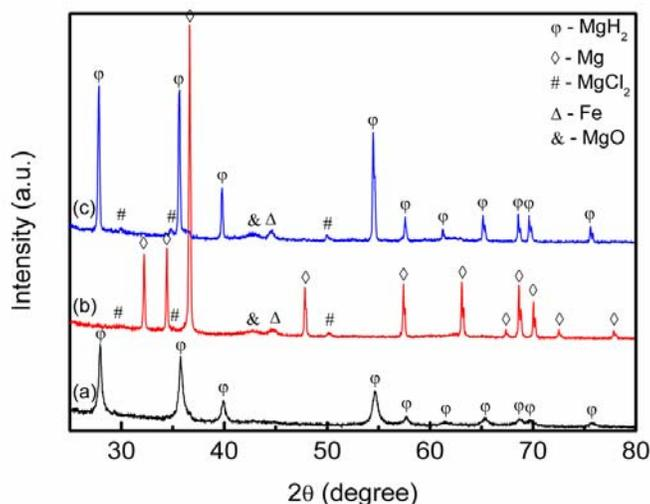
Fig. 7. X-ray diffraction patterns of the  $\text{FeCl}_3$ -doped  $\text{MgH}_2$  (a) after milling, (b) after dehydrogenation, and (c) after rehydrogenation.
