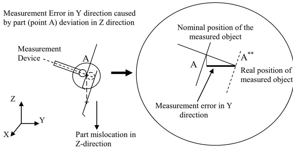
**Figure 5:** Illustration of the error in the  $Y$  direction caused by a part mislocation in  $Z$  direction.  $A$  – nominal position of the measurement point;  $A^*$  – mislocated position of the measurement point caused by part mislocation in  $Z$  direction;  $A^{**}$  – point measured. (Huang et al. 2004)
