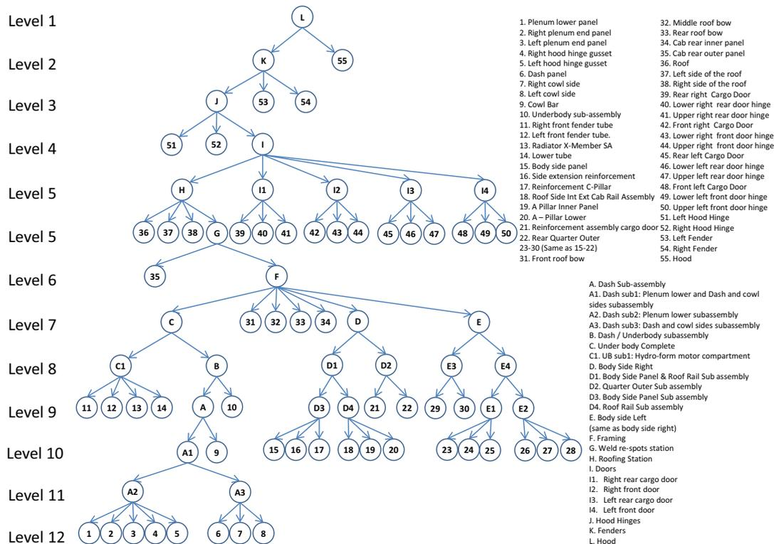
**Figure 1:** The process tree of a body-in-white
