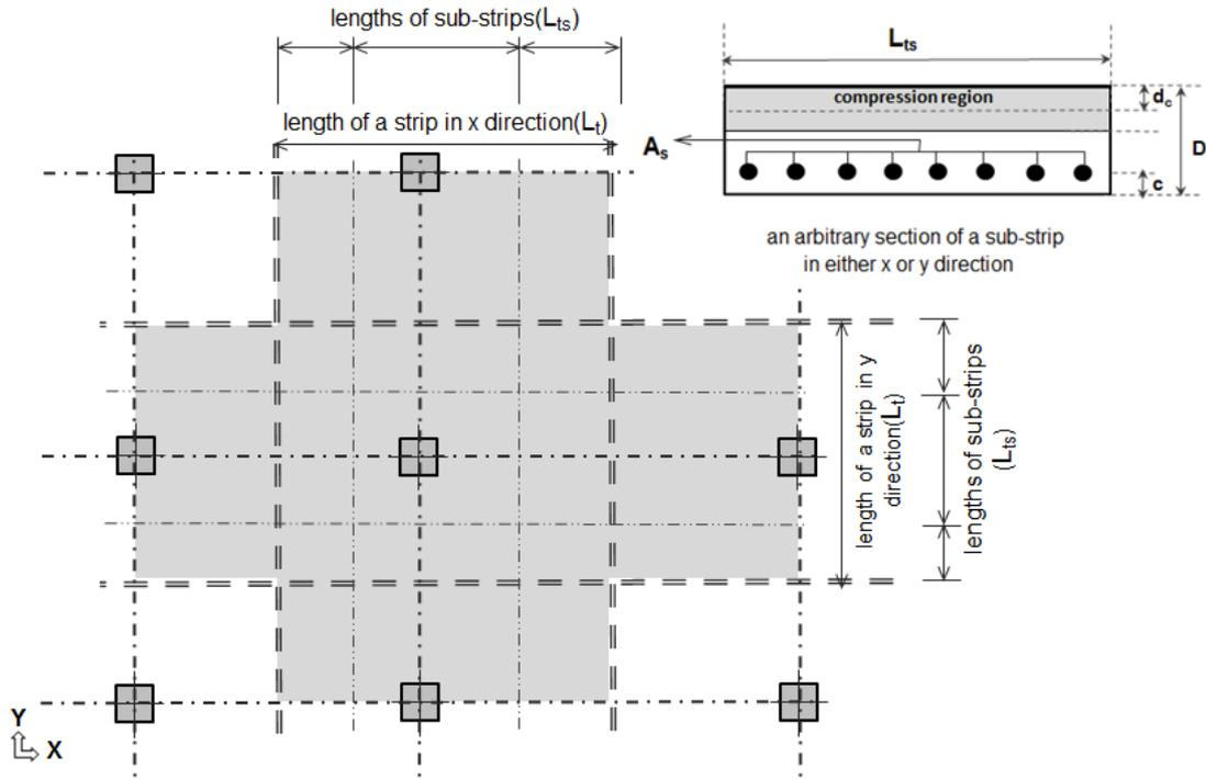
**Figure 1** Equivalent frame strips for flat plates
