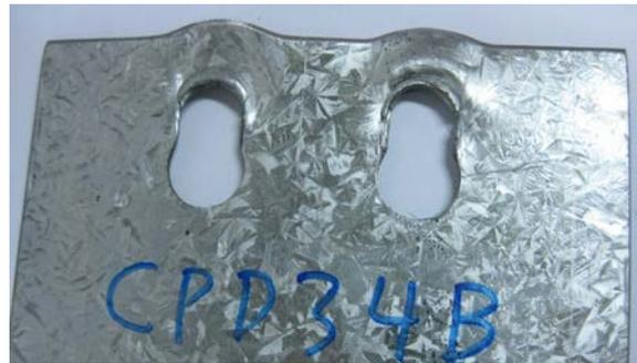
Figure 2. Shear-out of individual bolts
