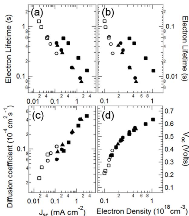
**Figure 3.** Electron lifetime versus (a)  $J_{sc}$ , or (b) electron density; electron diffusion coefficient versus (c)  $J_{sc}$ , and (d)  $V_{oc}$  versus electron density for DSSCs prepared with **P199** (circles), **P12** (triangles) and **P10** (squares). Measurements using reduced dye surface concentrations of **P199** (open circles) and **P10** (open squares) are also shown.
