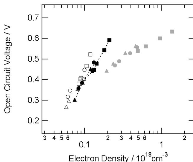
**Figure 5.**  $V_{oc}$  vs electron density for DSSCs using **P199** (circles), **P12** (triangles) and **P10** (squares) and containing Electrolyte **Ib** (grey, closed) with Electrolyte **II** (black, closed) and Electrolyte **III** (open).
