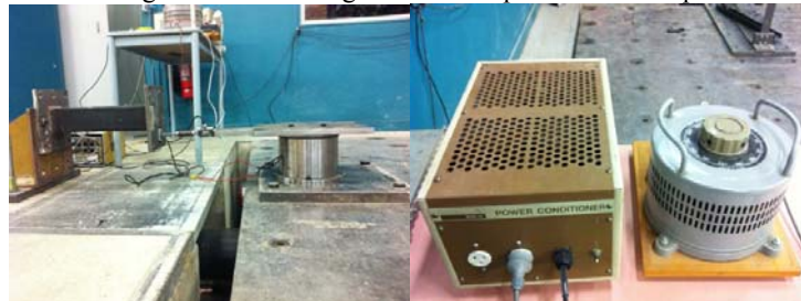
Figure 4. MRE seismic isolator during testing and equipments (power conditioner and the slider).
