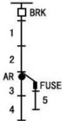
Fig. 3. Topology of a Simple Feeder with AR
