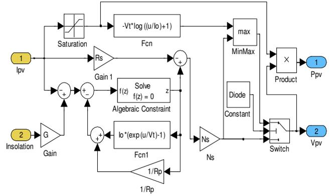
Figure 5. Simulink model of the PV module.
