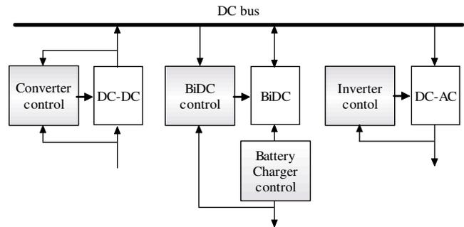
Figure 2. Control circuit of the PV BMS.
