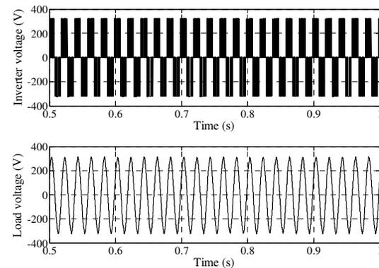
Figure 14. Inverter output voltage and load voltage.
