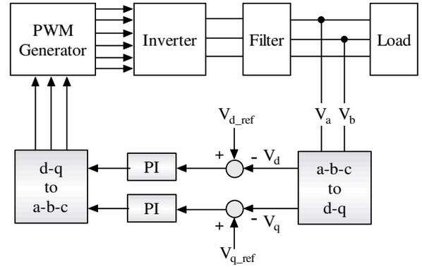
Figure 9. Vector control of inverter controller.
