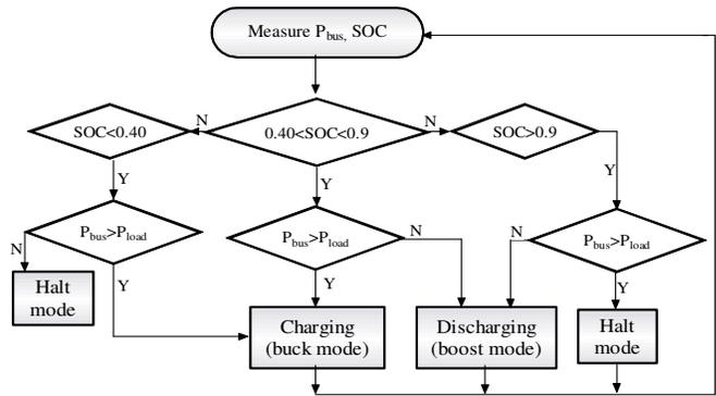
Figure 8. Bidirectional converter (battery charging/discharging) control algorithm.
