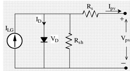
Figure 3. Equivalent circuit of PV module.
