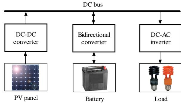
Figure 1. Power circuit of the PV BMS.
