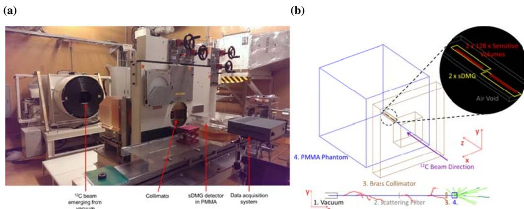
**FIGURE 2.** (a) sDMG detector embedded in PMMA phantom and with data acquisition system placed in experimental beamline, (b) schematic visualization of beamline from Geant4<sup>16-18</sup> simulation.
