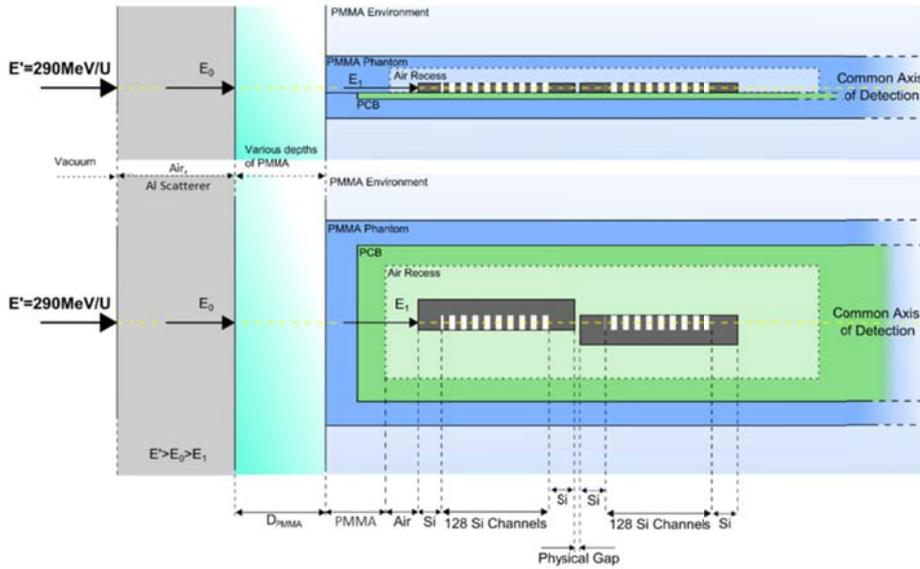
**FIGURE 3.** Detailed geometry of the sDMG in PMMA phantom for measurement of pristine Bragg peak (PBP) depth profile. The air void has an area  $19 \times 205$  mm relative to the beams eye view; 6 mm of air is between the phantom wall and first silicon wafer of the detector and the physical gap between two wafers is 0.6 mm.
