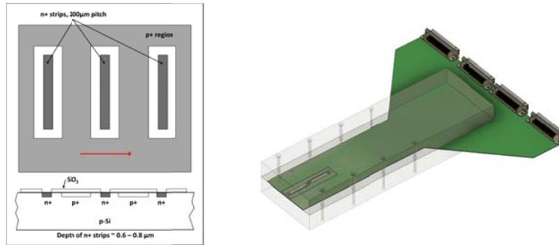
**FIGURE 1.** Schematics of the serial Dose Magnifying Glass (sDMG) comprised of two linear arrays detectors is wire bonded to a thin printed circuit board (PCB), the single axis of detection is indicated by the arrow.
