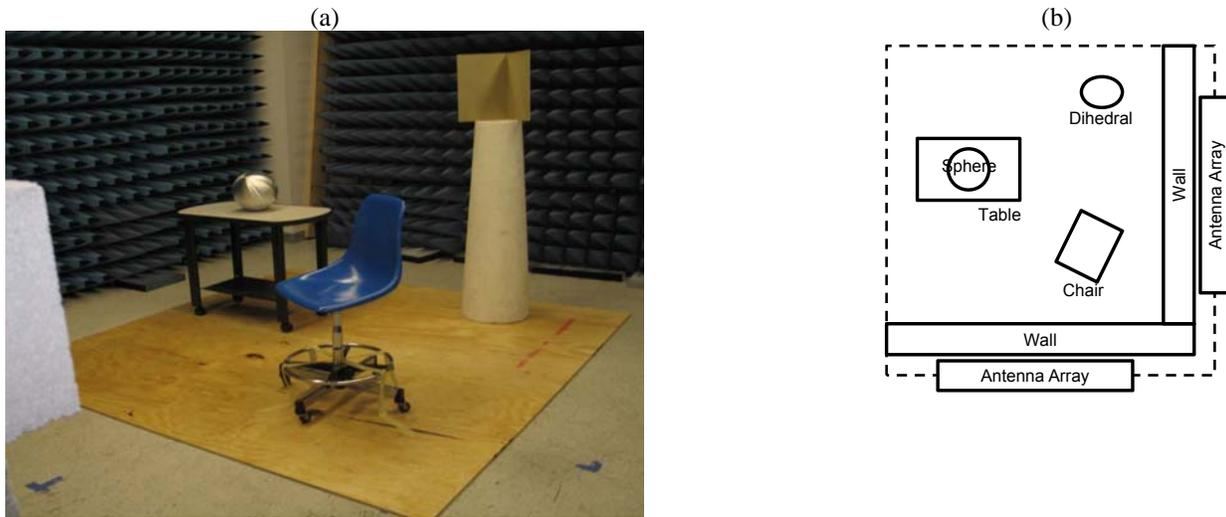
Fig. 6. The populated scene: (a) the scene is imaged through a homogenous concrete wall from two vantage points; (b) the schematic diagram of the scene.
