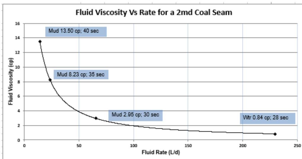
Figure 6: Relationship between viscosity and injection rates for a 2 md Coal Seam
