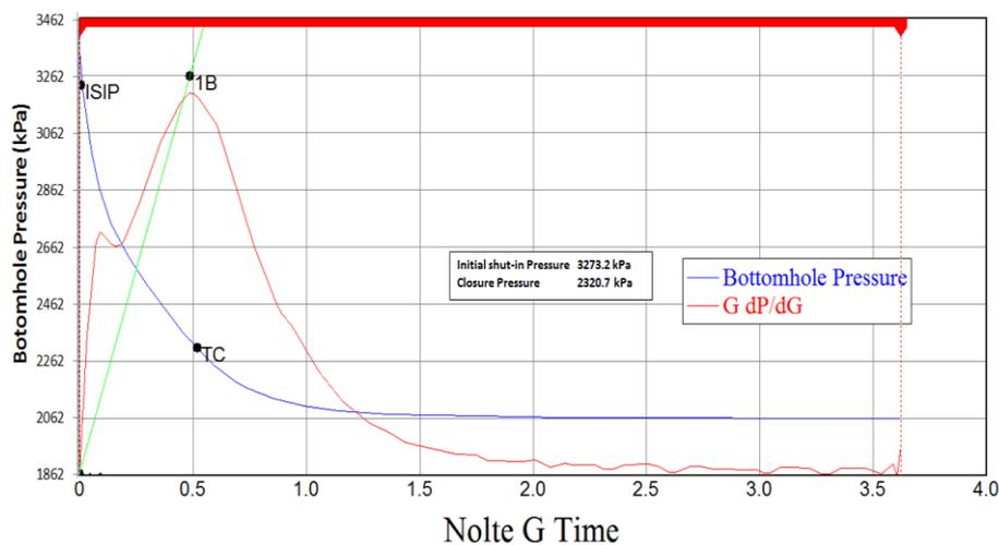
Figure 3: Coal closing pressure determination
