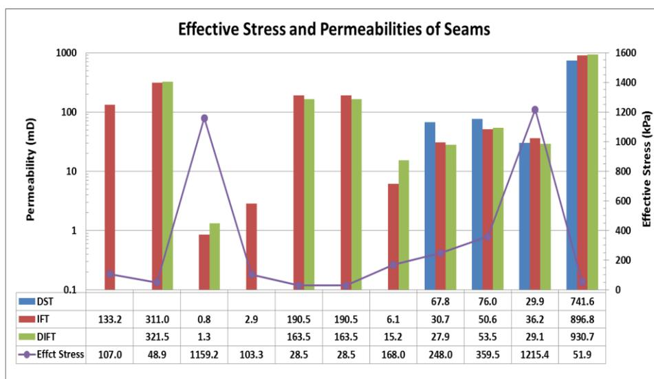
**Figure 7: An example of integration of field permeability and minimum stress**
