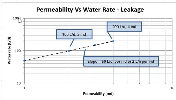
Figure 4: Possible errors due to a HQ test string leakage of 2 L/h
