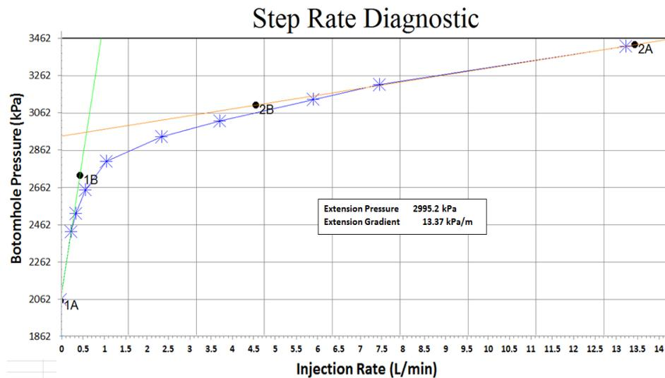
Figure 2: Step rate test of coal seam, with estimation of Fracture Extension Pressure
