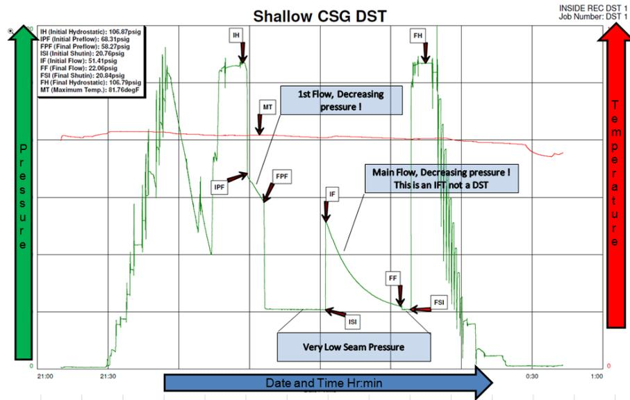
Figure 1: Results of a planned shallow CSG DST that is actually an IFT
