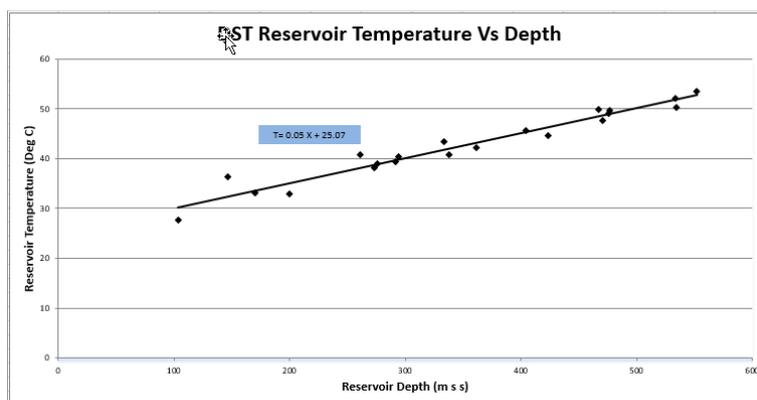
Figure 5: Field temperature gradient from DST measurements
