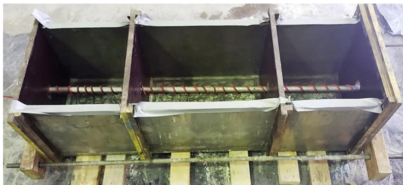
Figure 1: Concrete blocks casting assembly
