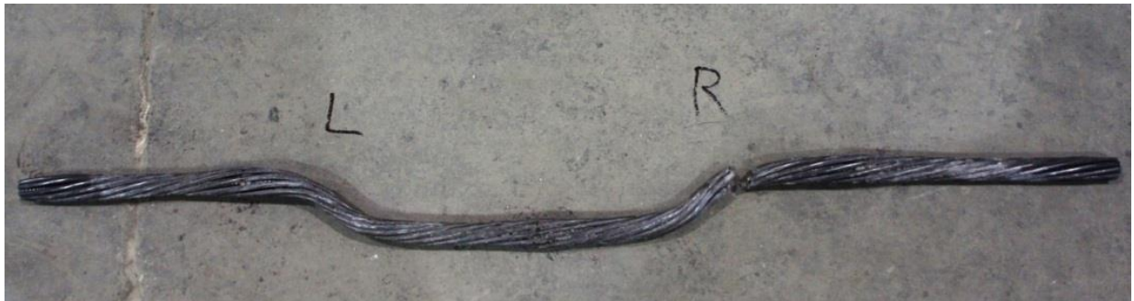
Figure 6: Failure angle of cable bolt
