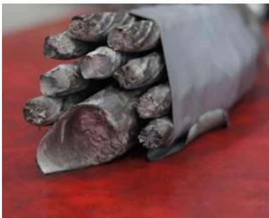
Figure 7: Tensile and shear failure of cable bolt
