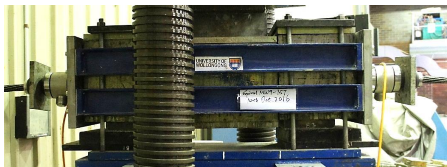
Figure 2: Double shear assembly without friction between concrete blocks
