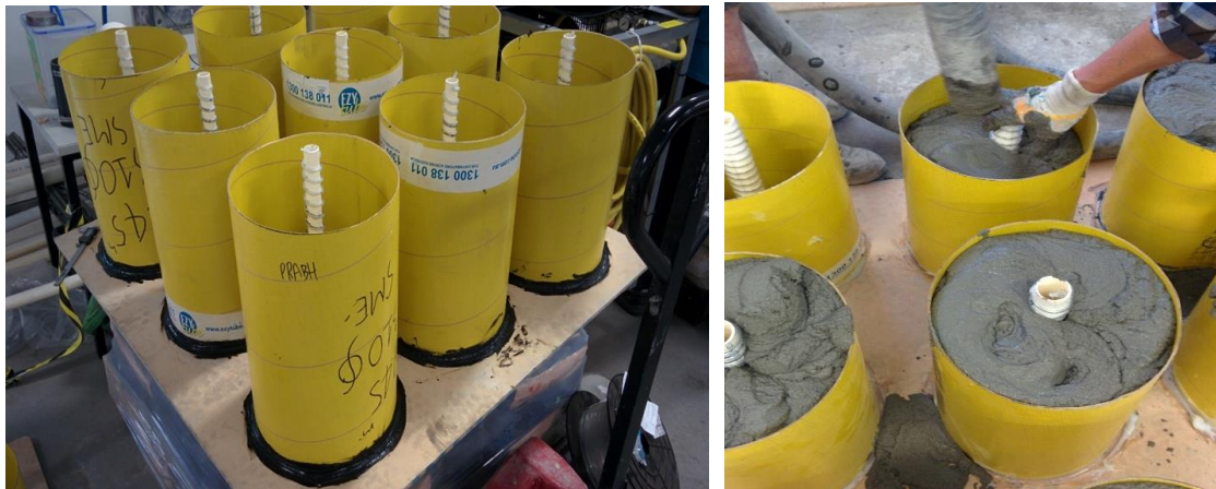
Figure 4: Prepared moulds to create the test samples (left) and pouring of cement mixture into moulds (right)
