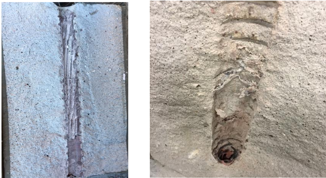
Figure 7: Dominant failure mode was between the grout and cable bolt (left) except in one 52 mm sample where failure occurred at the rock/grout interface (right)
