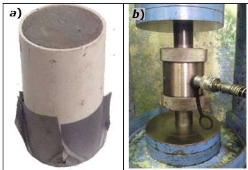
Figure 6: a) PVC mould containing prepared sample b) Triaxial cell in testing arrangement
