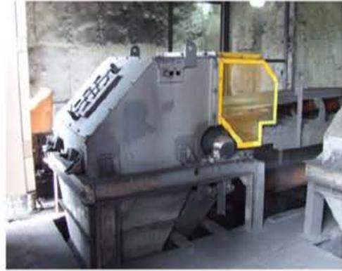
Figure 4: Coal Staithe Conveyor Belt Drive Pulley
