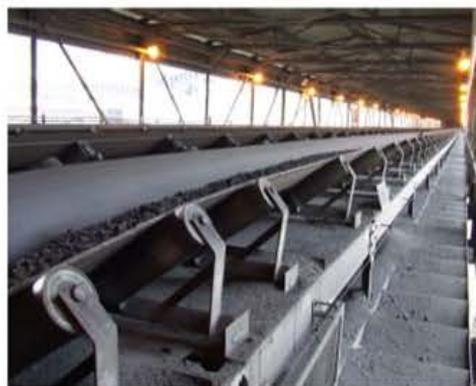
Figure 3: Inclined Conveyor from Coal Bunker
