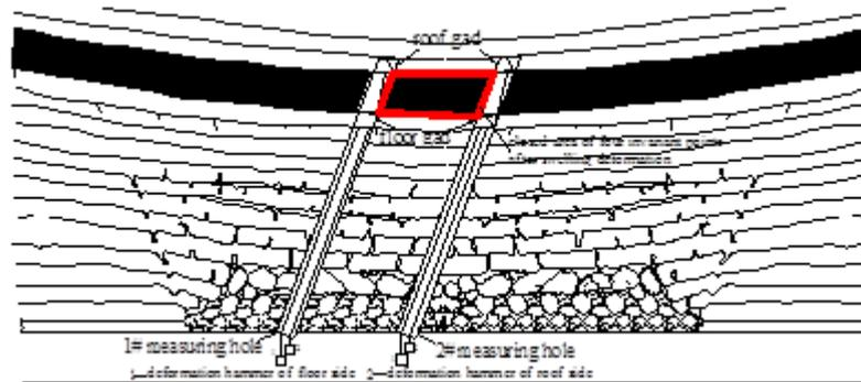
Figure: 3 Schematic diagram of measuring hole layout
