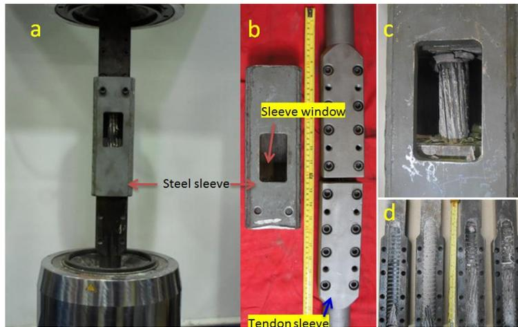
Figure 4: Axially split double embedment pull testing apparatus
