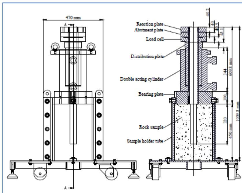
Figure 2: UNSW LSEPT pull testing apparatus (Chen *et al.*, 2014)
