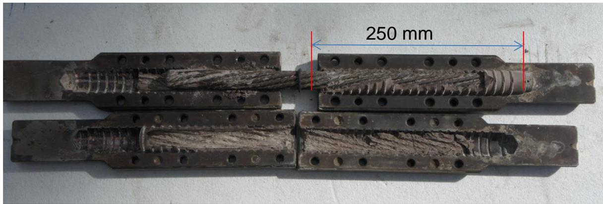
**Figure 6: Post-test two halves of the pull out apparatus with encapsulated cable bolt**
