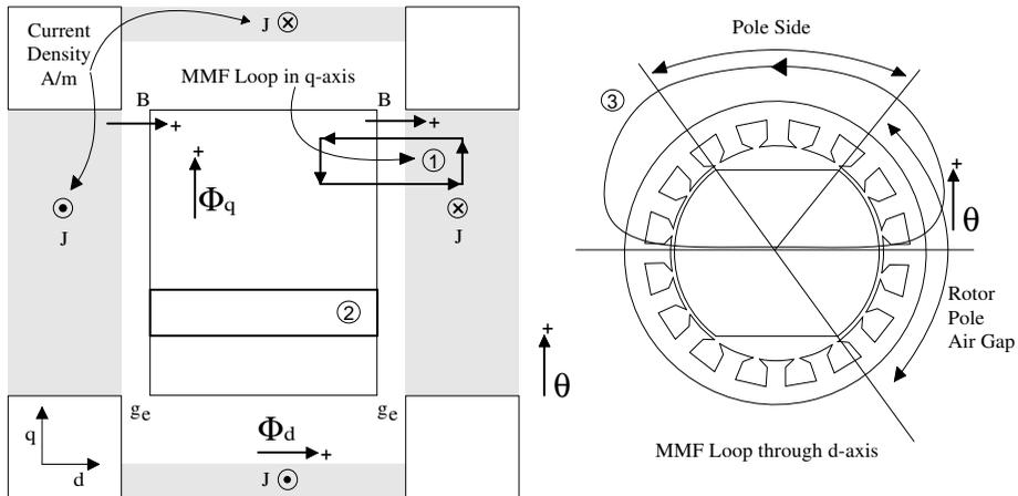
Figure 5: Machine Model
