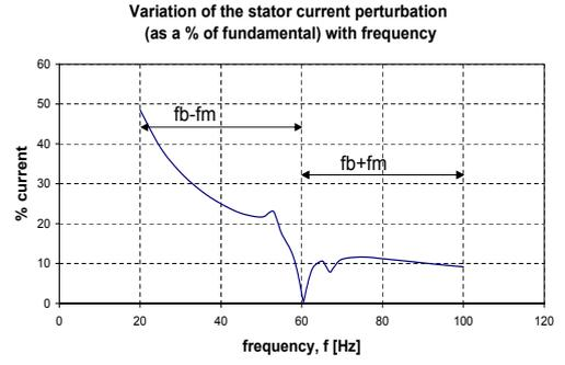
Figure 4: Variation of stator current perturbation (as a percentage of steady state current) ( $\Delta i_{as}$ ) with frequency of the injected voltage perturbation ( $f$ );  $f = f_b - f_m$  or  $f = f_b + f_m$
