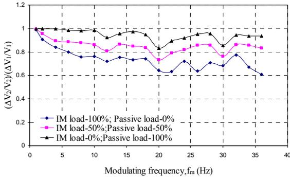
**Figure 7:** Variation of flicker transfer from upstream to downstream for different load compositions
