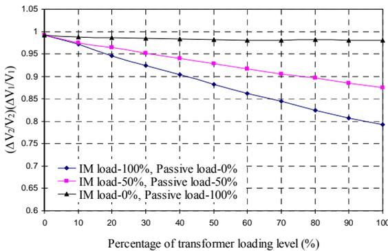
**Figure 8:** Variation of upstream to downstream flicker transfer for different loading levels
