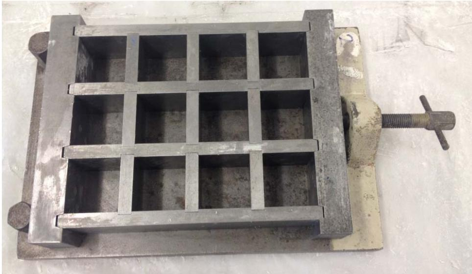
**Figure 1: Steel mould assembly of 40 mm cubes**
