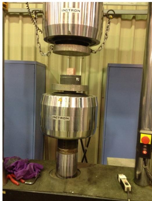
Figure 3: Compression strength – test setup
