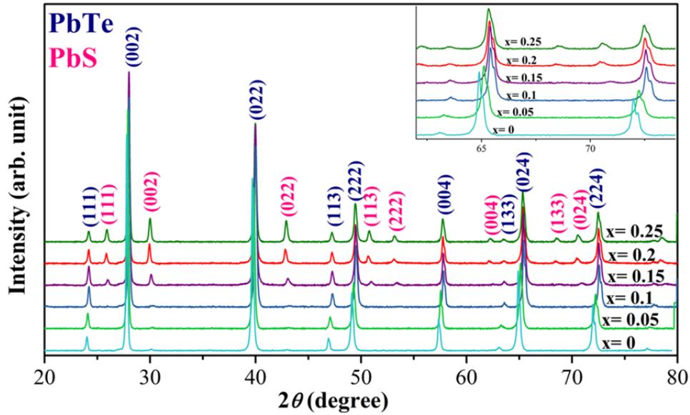
**Figure 1.** Room temperature X-ray diffraction patterns for  $(\text{PbTe})_{(0.9-x)}(\text{PbSe})_{0.1}(\text{PbS})_x$  ( $x = 0, 0.05, 0.1, 0.15, 0.2$  and  $0.25$ ) alloys. The inset shows shifting of diffraction peaks to higher angles for  $x$  up to  $0.1$  due to the alloying effect.
