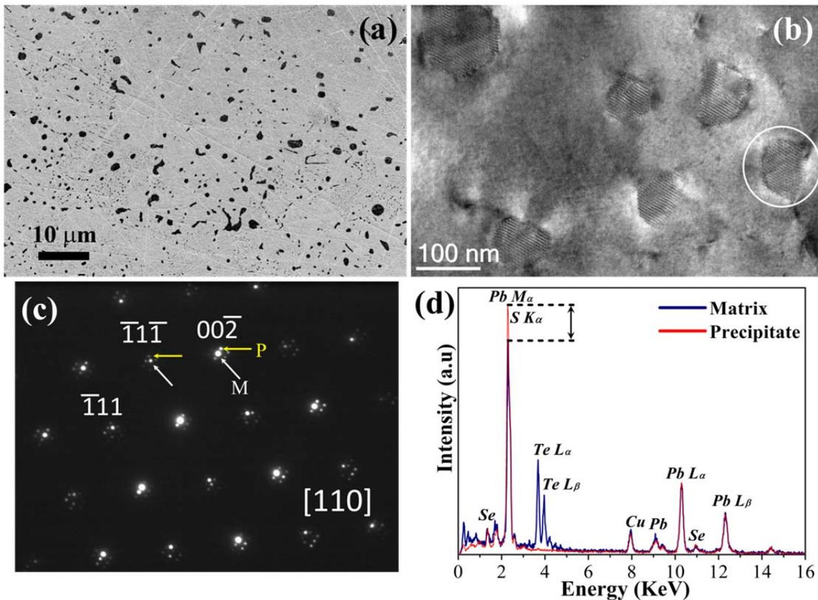
**Figure 2.** (a) SEM image of sintered  $(\text{PbTe})_{0.75}(\text{PbSe})_{0.1}(\text{PbS})_{0.15}$  (S15) sample, showing the morphology and the distribution of precipitates in the matrix, the sample has been through several cycles of heating up to  $850$  K and cooling during transport properties measurements; (b) Bright field TEM micrograph of sulphur-rich precipitates in the tellurium-rich matrix
