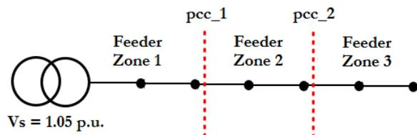
Fig. 1: Single Line Diagram 'Short' LV Feeder
