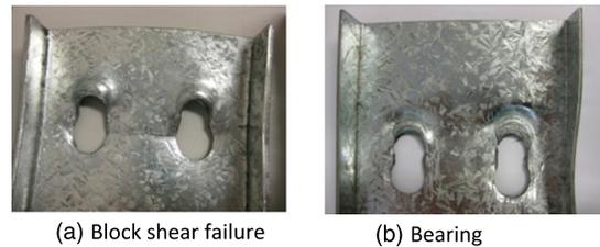
Fig. 3. Failure modes with only a single row of bolts: (a) block shear; (b) bearing
