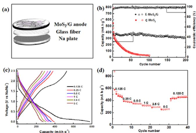
**Figure 2.** Electrochemical performances of half cells: (a) schematic structure of sodium-ion battery; (b) cycling performances of C-MoS<sub>2</sub> and MoS<sub>2</sub>/G composite at 100 mA g<sup>-1</sup> (0.25 C); and coulombic efficiency of MoS<sub>2</sub>/G composite; (c) charge/discharge curves and (d) rate capability of MoS<sub>2</sub>/G at various current rate.
