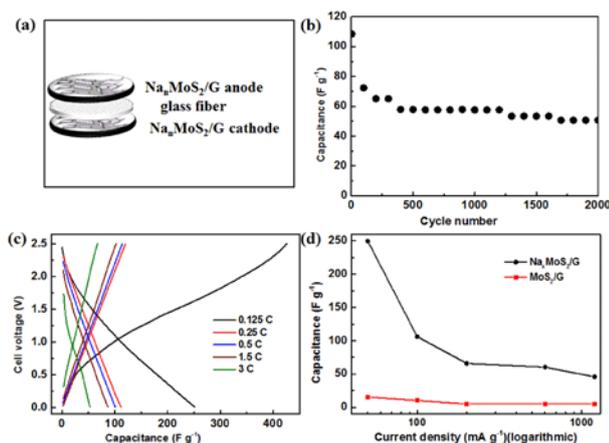
**Figure 3.** Electrochemical performances of full cells: (a) schematic structure of sodium-ion pseudocapacitor; (b) capacitance of NICs at 1.5 C with prolonged cycling; (c) charge/discharge curves of NICs at various current rates; (d) comparison of capacitance between MoS<sub>2</sub> NICs and Na<sub>n</sub>MoS<sub>2</sub> NICs at various current rates
