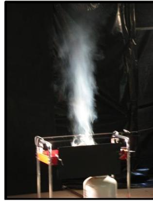
**Figure 4 - Typical smoke plume resulting from heating the coal and grease fuel mixture**
