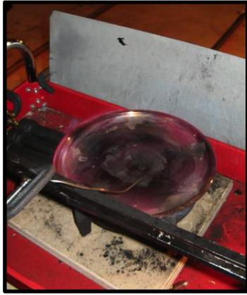
**Figure 3 - Heated simulated bearing housing without fuel**
