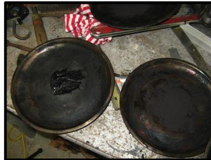
Figure 2 - Simulated bearing housings with surface coal and grease
