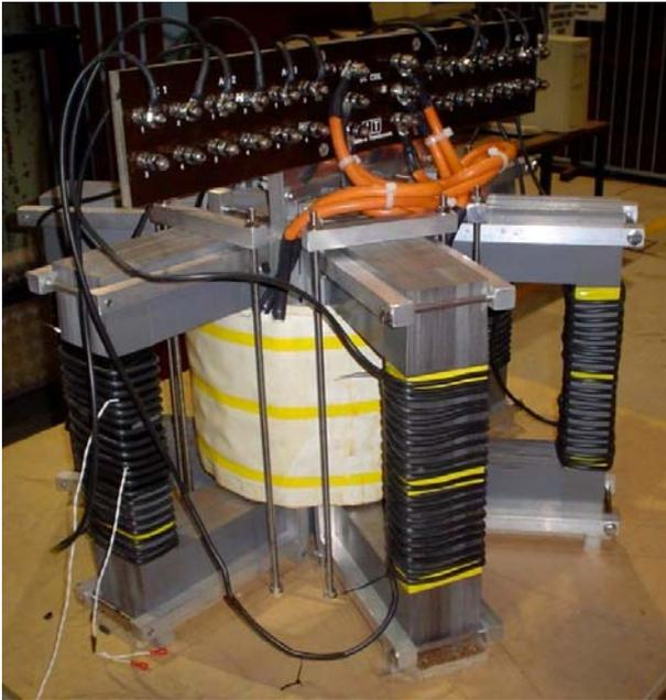
Figure 3. Prototype 3-Phase FCL
