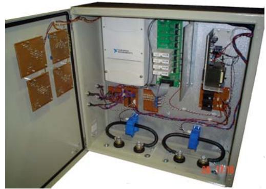
Figure 5. Test System DAQ and Sensor Enclosure
