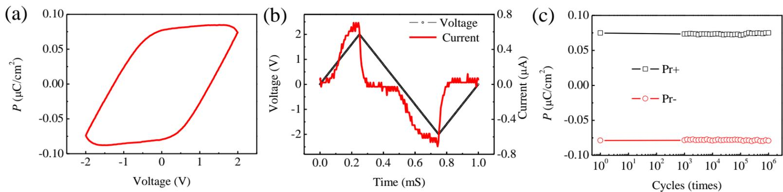
Fig. 3 (a) Electrical hysteresis loop of SmFeO<sub>3</sub> film on STO:Nb at room temperature, (b) time dependence of applied voltage and corresponding current, (c) fatigue test results after 10<sup>6</sup> cycles (10 data points every decade).
