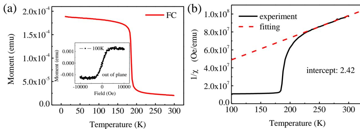
Fig. 6 (a) Temperature dependence of magnetic moment from 10 K to 300 K, and magnetic hysteresis loop measured at 100 K (inset); (b) antiferromagnetic interaction of  $\text{Fe}^{3+}$  sublattice confirmed by Curie-Weiss law fitting with temperature range from 100-300 K.
