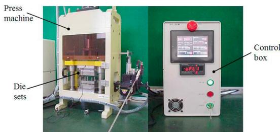
Fig. 4. Desk-top servo press machine DT-3AW.
