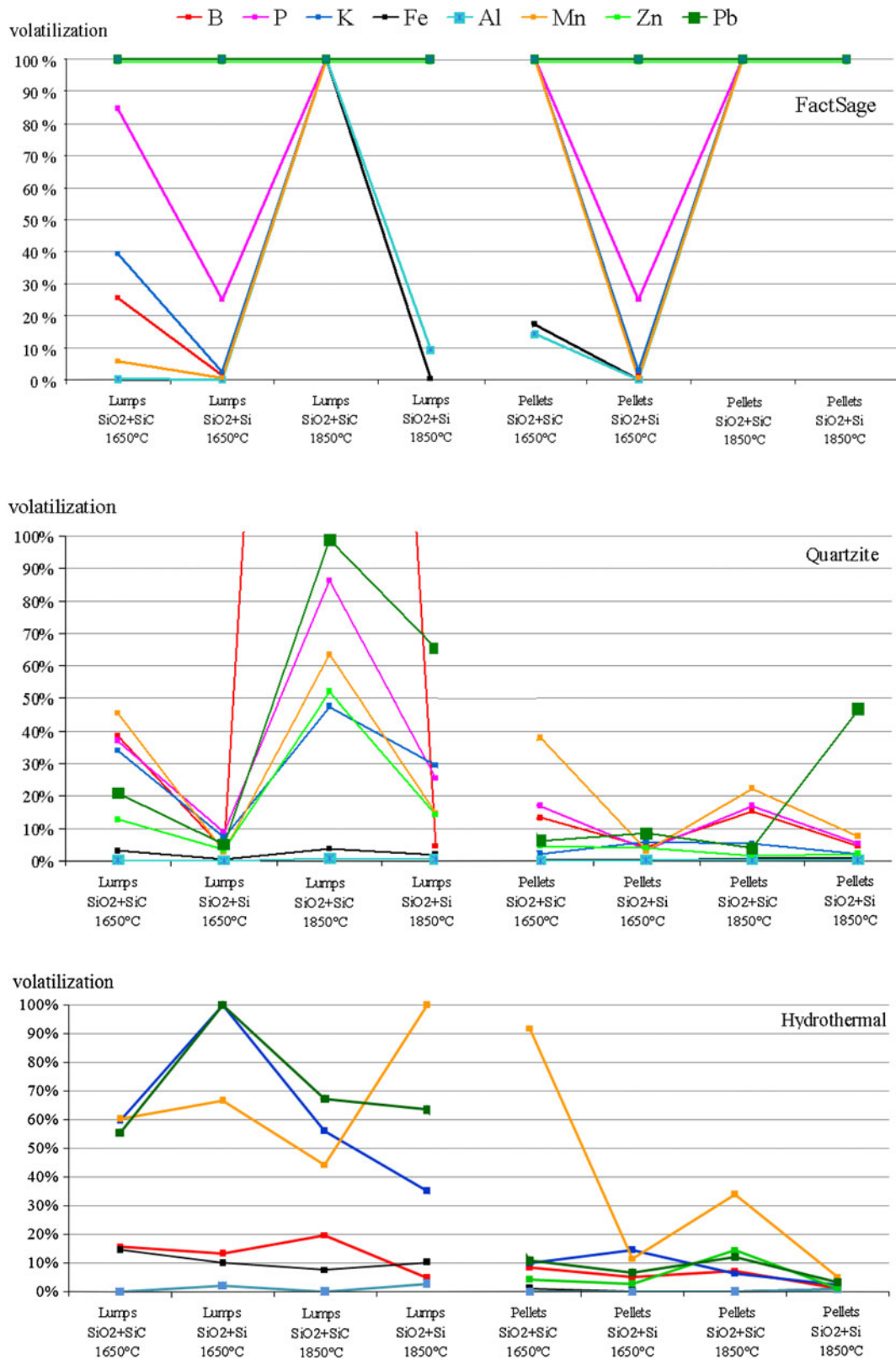
Fig. 4—Volatilization of elements in mass pct shown for different charge types, mixes and temperatures. Top to bottom: thermodynamic calculations, quartzite, and hydrothermal quartz. The volatility of P and Zn are not shown for all the experimental conditions in hydrothermal quartz because of the high concentration of these elements in the blank used as analytical reference.
