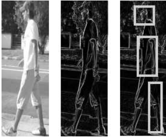
Fig. 1. Left: an image window. Middle: the edge magnitude. Right: three edge density features where each feature is the average edge magnitude in a specific subregion.
