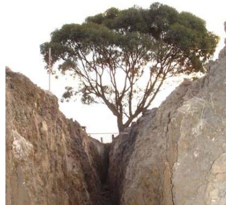
Figure 4. A photograph of the excavated trench to observe the tree root pattern and distribution.
