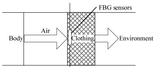
Fig. 7. Heat transmission model between body and clothed FBG sensors.
