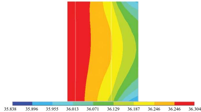
Fig. 10. Predicting temperature distribution in intelligent clothing using ANSYS.
