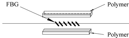
Fig. 1. Sketch of polymer package for FBG.
