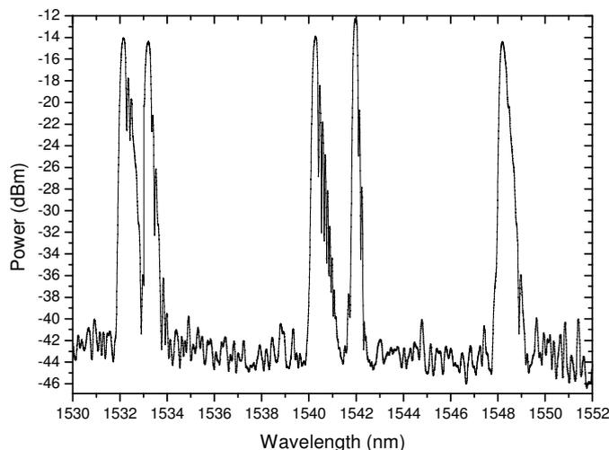
Fig. 6. Spectrum of five series polymer-packaged FBG sensors.
