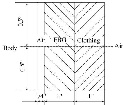
Fig. 9. Temperature finite element model for intelligent clothing.
