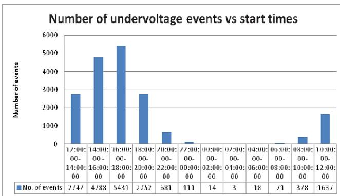
Figure 4 -Number of undervoltage events versus start times
