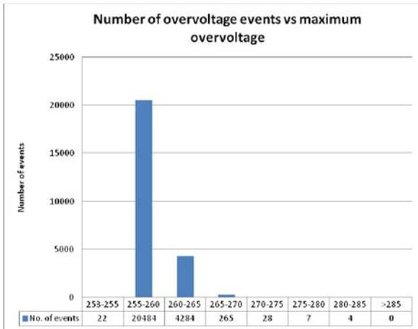
Figure 10 - Number of overvoltage events versus highest voltage
