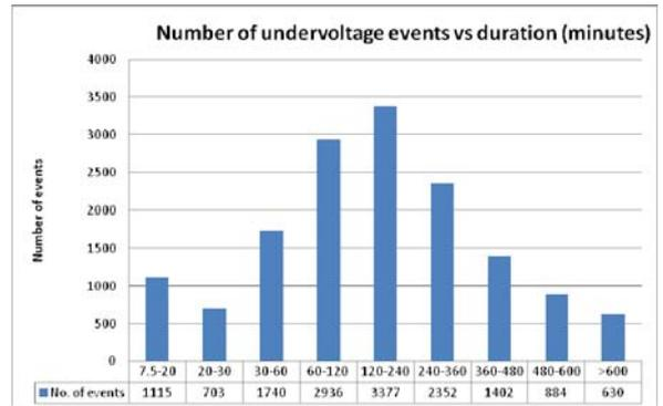
Figure 5 - Number of undervoltage events versus duration (minutes)
