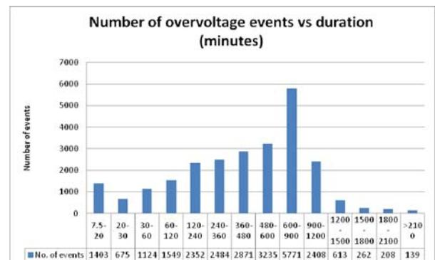
Figure 9 - Number of overvoltage events versus duration (minutes)
