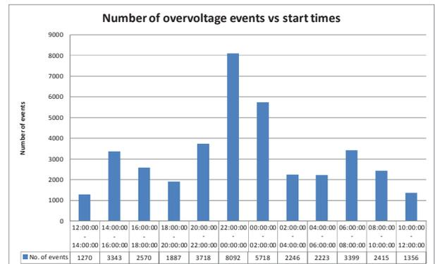
Figure 8 - Number of overvoltage events versus start times
