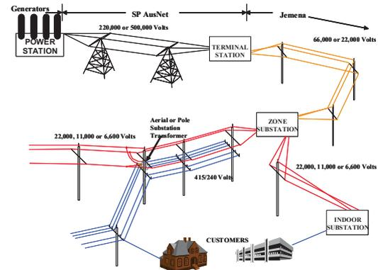
Figure 1 - Typical Electricity Supply System in Victoria, Australia
