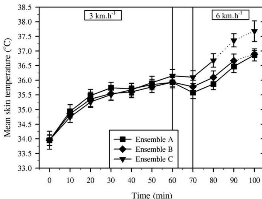
**Figure 2:** Mean skin temperatures during steady-state work in a temperate environment whilst wearing three different CBR ensembles. Broken lines indicate times where subjects terminated a trial prematurely. Data are means with standard errors of the means.
