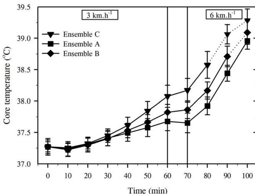
**Figure 3:** Rectal temperatures during steady-state work in a temperate environment whilst wearing three CBR ensembles. Broken lines indicate times where subjects terminated a trial prematurely. Data are means with standard errors of the means.
